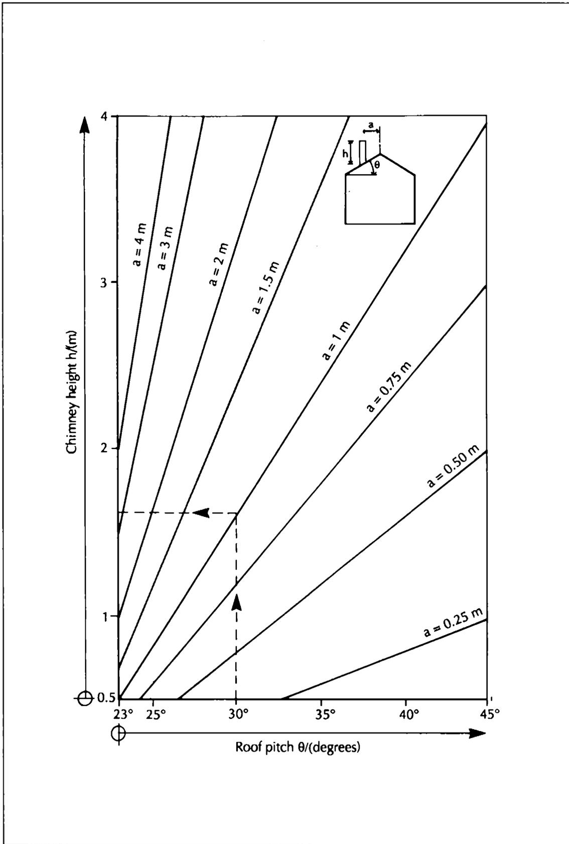
Figure 3.7 Location and Height of the Outlets of Natural Ventilation Ducts to Avoid Back-Draughting
