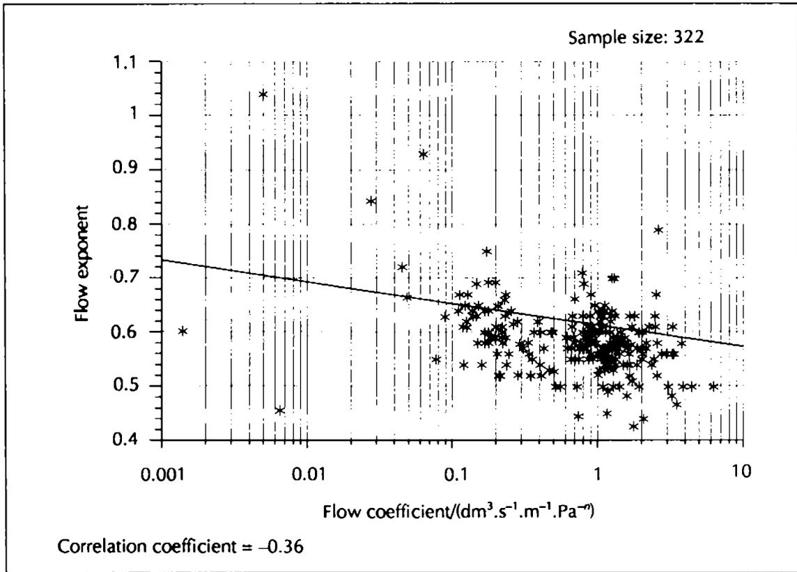
Figure 1.3 (a) Flow per Unit Length of Crack
