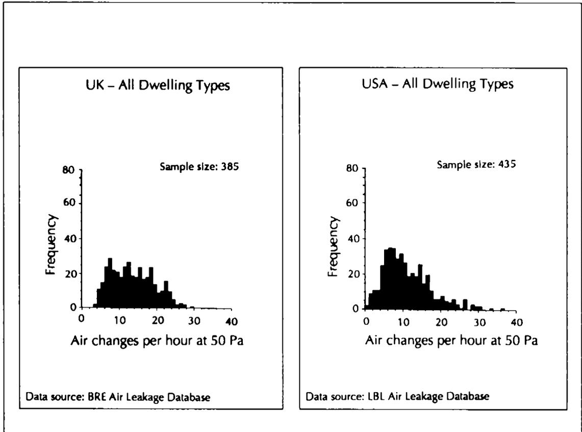
Figure 2.4 Comparison of Whole Building Leakage Values at 50 Pa
