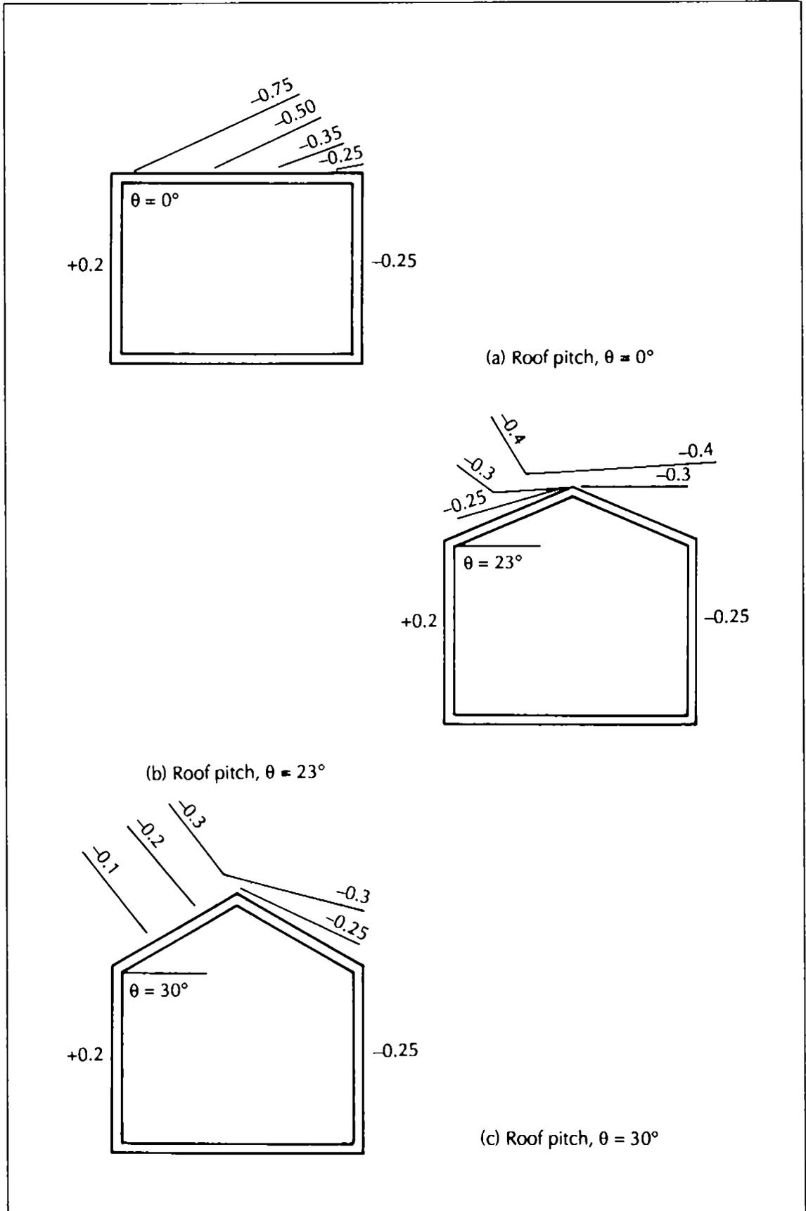
Figure 3.6 Wind Pressure Coefficients for Protrusions above Roof Level
