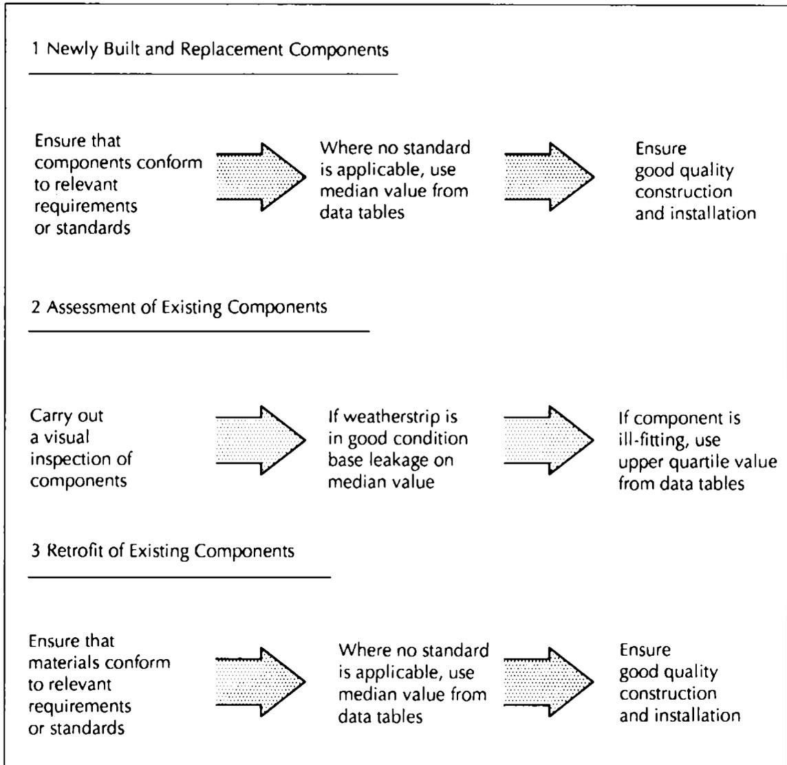
Figure 1.2 Application of Air Leakage Data
