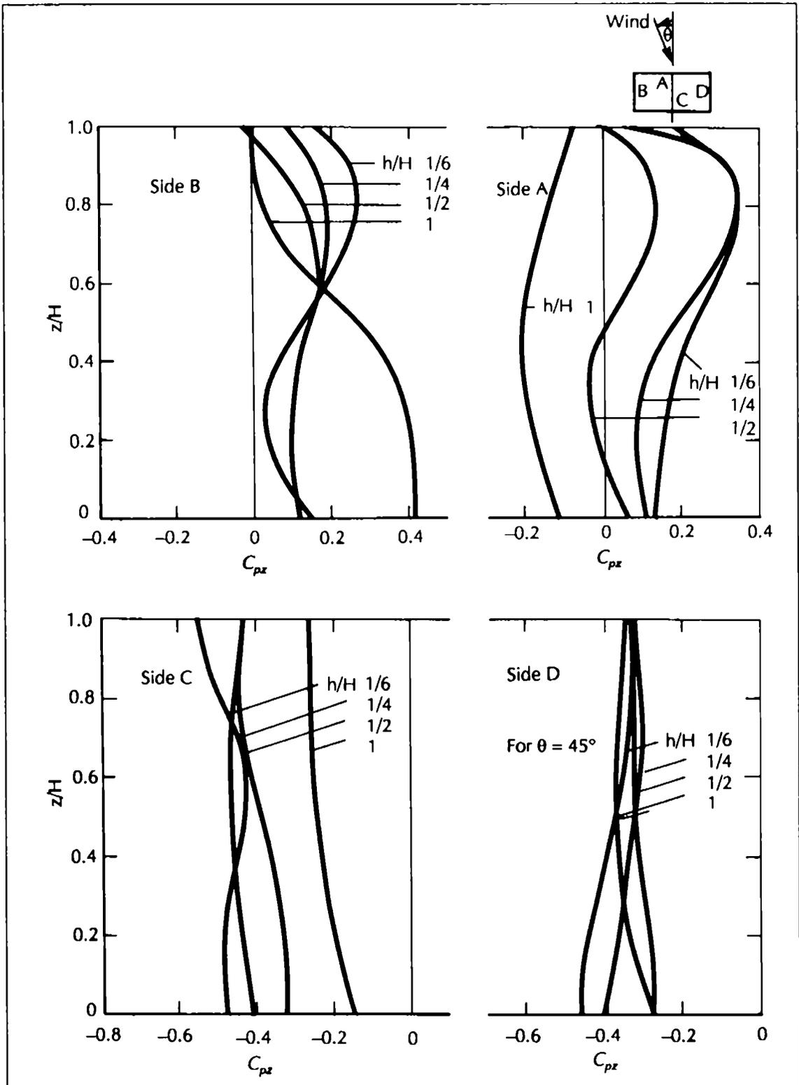
Figure 3.4 (i) Vertical Distribution of Weighted Mean Wind Pressure Coefficients  $C_{pz}$  for Various Surrounding Obstruction Heights (Wind Angle  $45^\circ$ )
