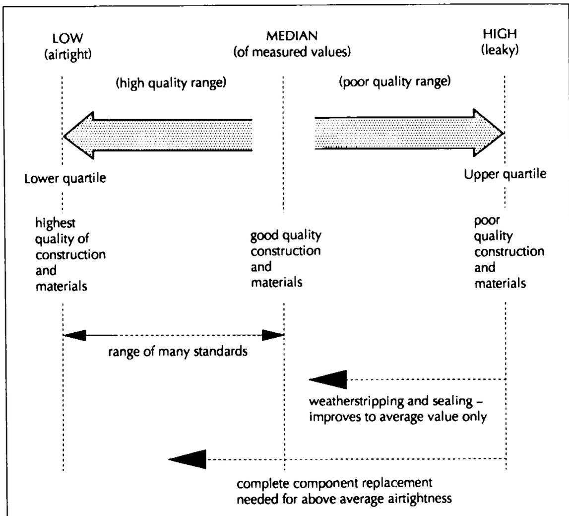
Figure 1.1 Air Leakage of Components
