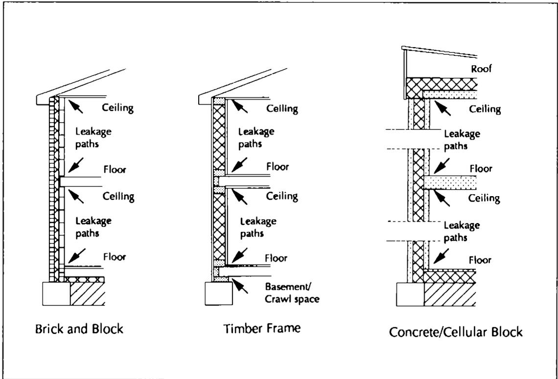
Figure 1.8 Floor/Wall/Ceiling Joints
