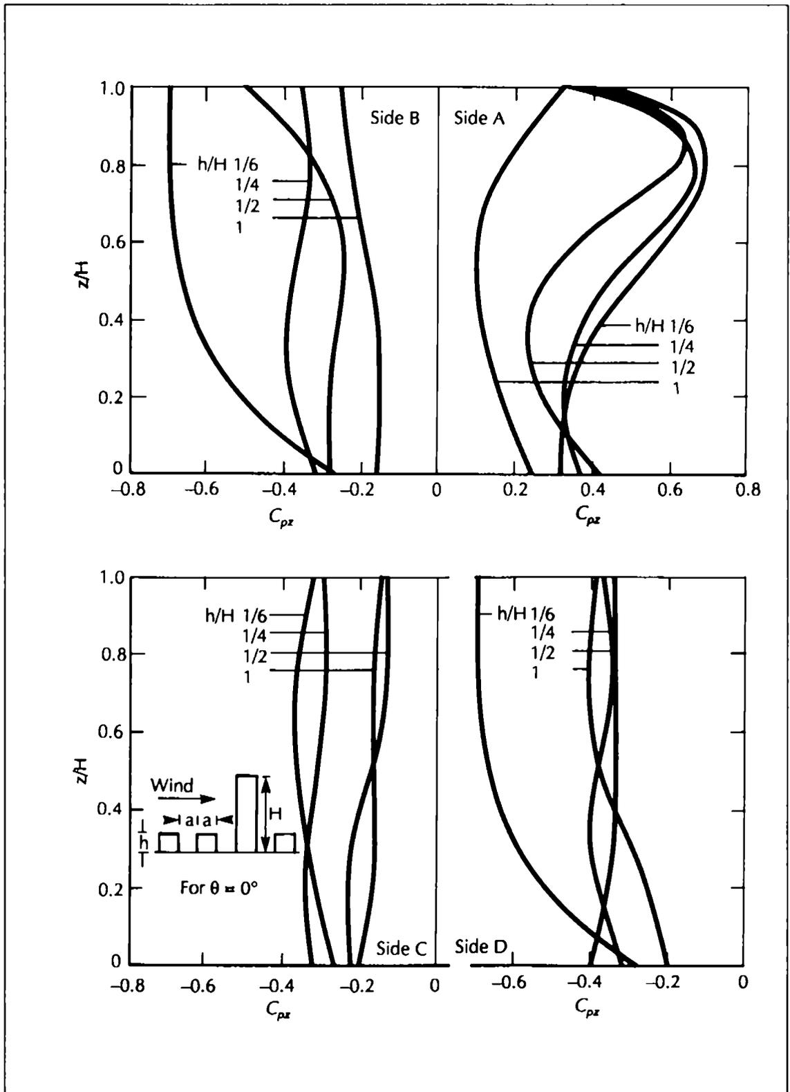
Figure 3.4. (ii) Vertical Distribution of Weighted Mean Wind Pressure Coefficients  $C_{pz}$  for Various Surrounding Obstruction Heights (Wind Angle  $0^\circ$ )
