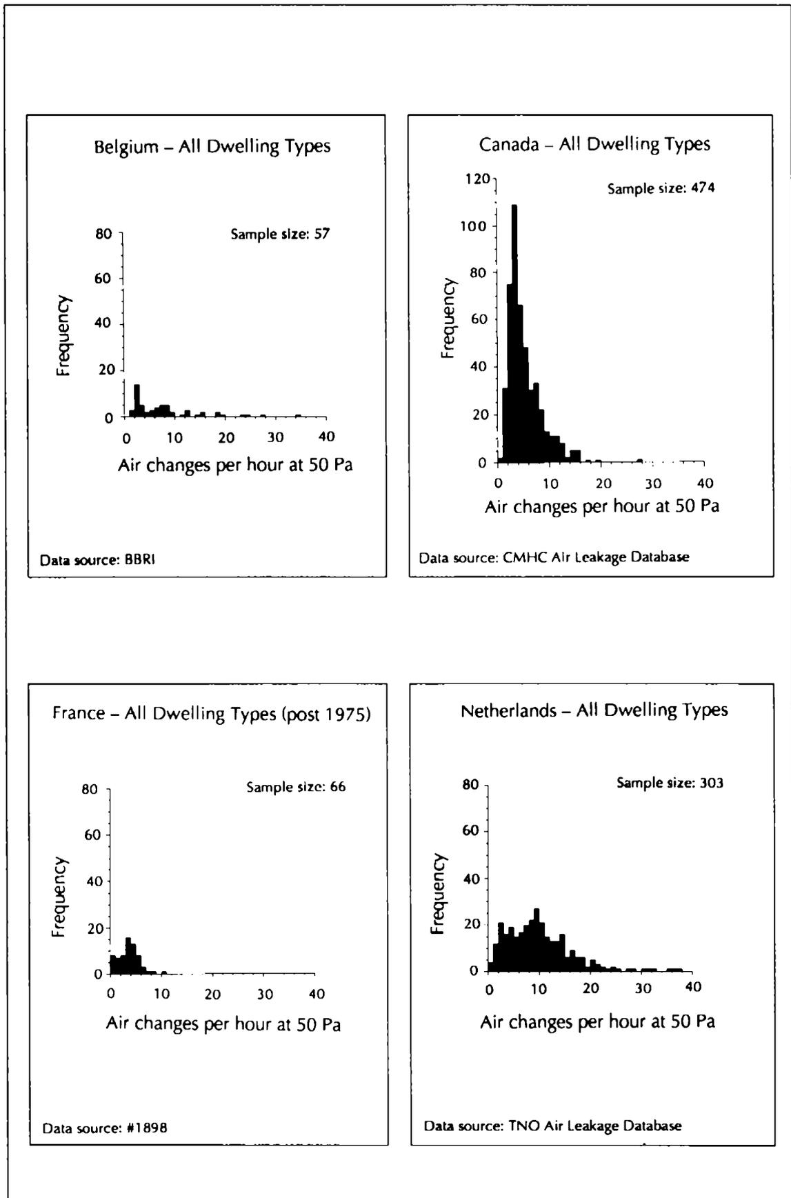
Figure 2.4 Comparison of Whole Building Leakage Values at 50 Pa
