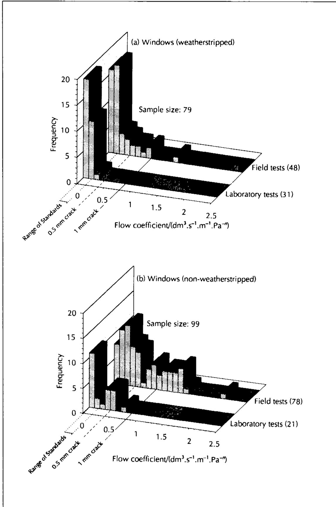
Figure 1.4 Air Leakage Distributions for Windows
